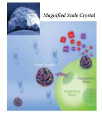
Inside the Centurion system are thousands of tiny Anti-Scale beads. Atomic level templates on the surface of the beads act as catalysts causing the calcium, and bicarbonate ions in hard water to form microscopic crystals.
