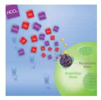
Once the crystals grow to a certain size they are released from the bead. The crystals in solution keep the hardness out of the water so that it can't deposit and form scale on the plumbing surfaces or interfere with soaps and detergents.
